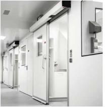
The hermetic sliding door from Gilgen automatically creates a seal for your rooms, preventing the unwanted exchange of air, impurities and other contaminants. When the door is closed, the pivot mechanism in the drive unit lowers the door leaf and presses it against the door frame. In combination with the sealing gaskets, this lowering movement ensures that the door creates a hermetic seal.
